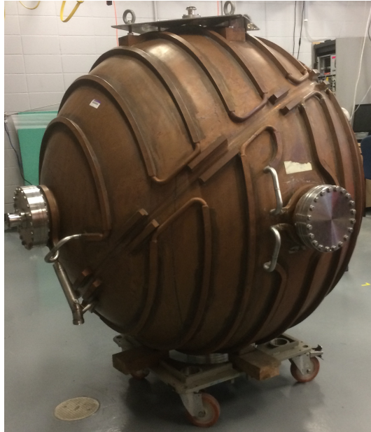
Figure 3.17: Accelerating cavity from LEP converted into SPC.
