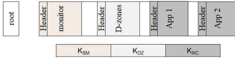
Figure 5-10: This figure presents the keys used to compute the hash to verify the integrity of each application.
