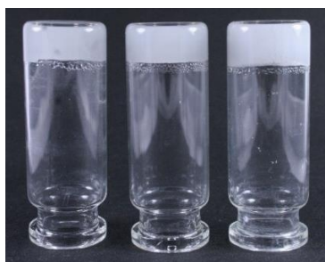
Figure I-18: Alkylaldonamide gels obtained after cooling down of the hot solutions.
