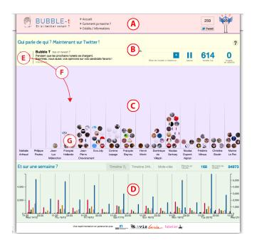
Figure 5.4: Bubble-T visual components: A. A header, B. A control Bar, C. A realtime visualization, D. Day and week time frame visualizations, E. Tweets read area incomming token appear here, F. An example of the trajectory of a tweet, G. A column containing a set of tweets. (Screenshot from the original website 21/12/2011).
