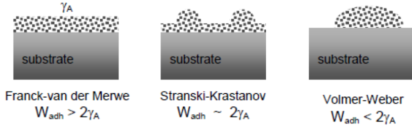
Figure 2.38: Film growth modes according to the criterion of adhesion/surface energies. The Frank van der Merwe mode corresponds to a layer-by-layer growth, the Stranski-Krastanov mode to growth of a continuous layer followed by 3D clusters and the Vomer-Weber mode is characteristic of 3D island growth.
