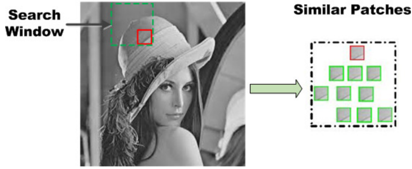
Figure 4.6: Search window of the NS model. The search window includes the area that is clean or already recovered.
