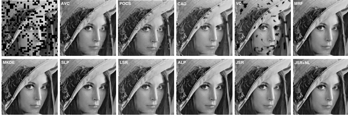
Figure 4.9: Subjective comparison between the proposed JSR+NL results and those of other EC techniques for random loss patterns with 30% PLR using Lena concealed image.
