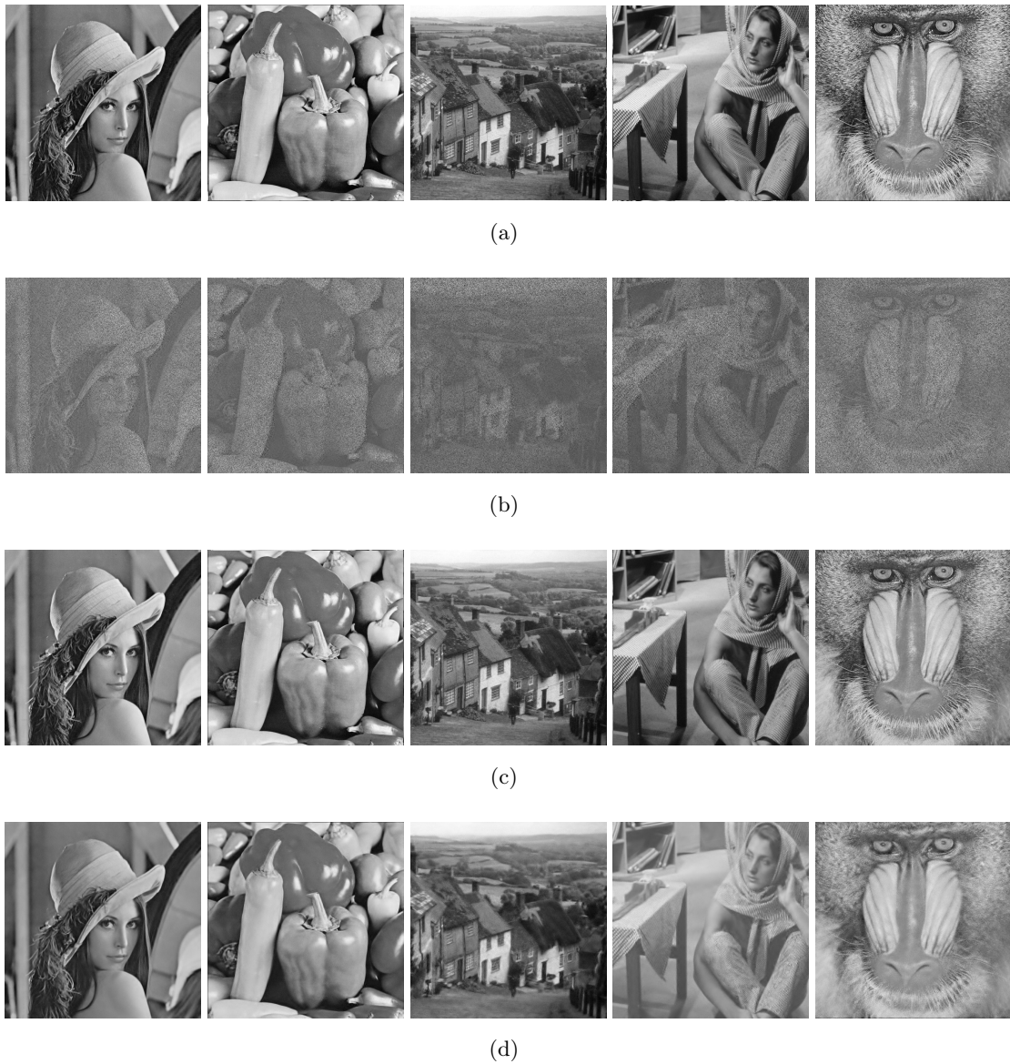
Figure 5.4: Subjective results for the test images. (a) Original image, (b) Received images with PLR = 30\% , (c) Concealed images with PLR = 30\% , (d) Concealed images with PLR = 70\% . From left to right: Lena , Peppers , Goldhill , Barbara , and Mandrill .
