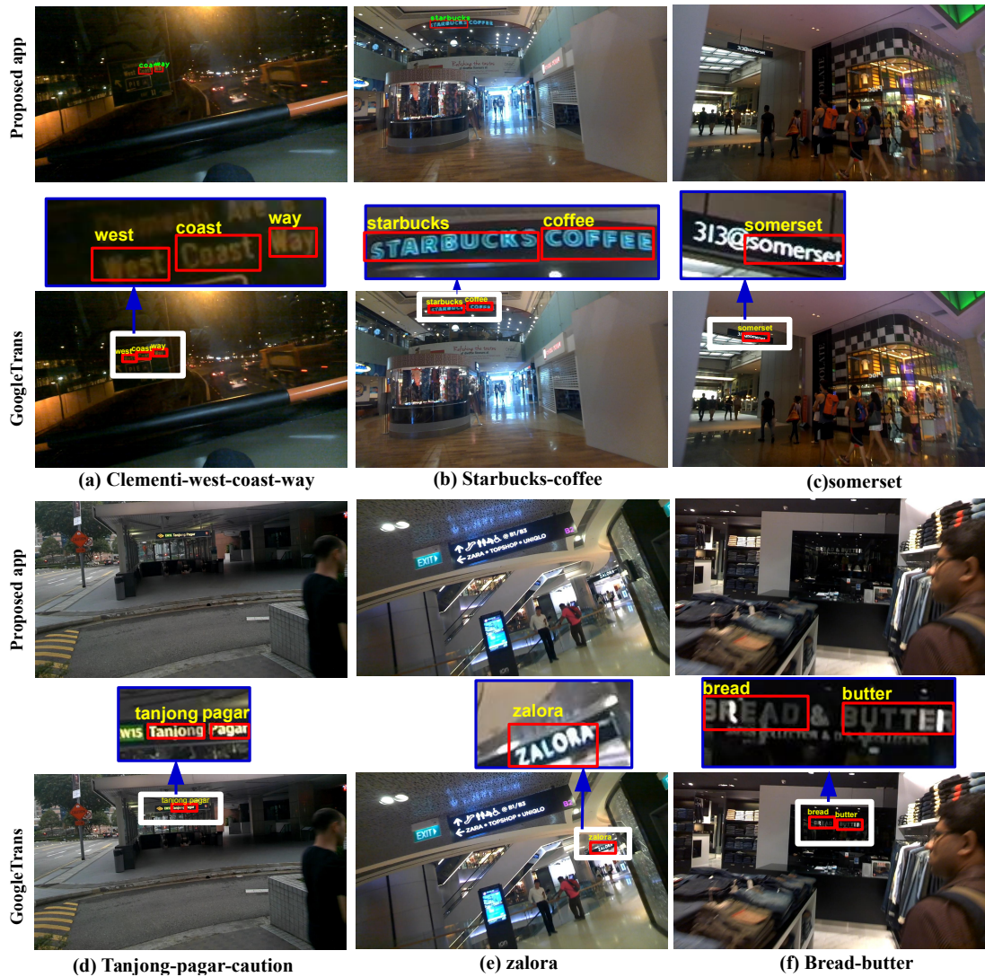
FIGURE 5.9 – Example images on which the GoogleTrans app provides better performance than the proposed app. The green recognized words are generated by the proposed app and the yellow recognized words are generated by the GoogleTrans. The white boxes describe from where images are cropped.
