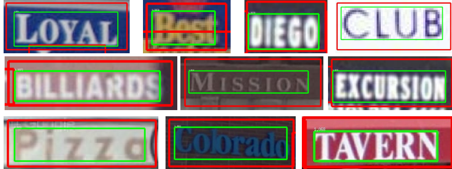
FIGURE 3.6 – There are some examples of the SVT ground truth boxes which our proposals cannot localize with the IoU threshold of 0.7. The red boxes are the ground truths and the green boxes are our proposals. The proposal boxes are much more smaller and closer to the scene text objects than the ground truth boxes.
