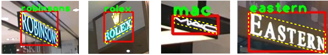
FIGURE 6.7 – Some examples of non-horizontal texts which have been detected successfully by the MPT scene text proposal technique while decided as miss detection in the IoU based evaluation. They are cropped out from images in the incidental scene text dataset. The red boxes are boxes generated by the MPT technique and the dash yellow boxes are ground truth bounding boxes.
