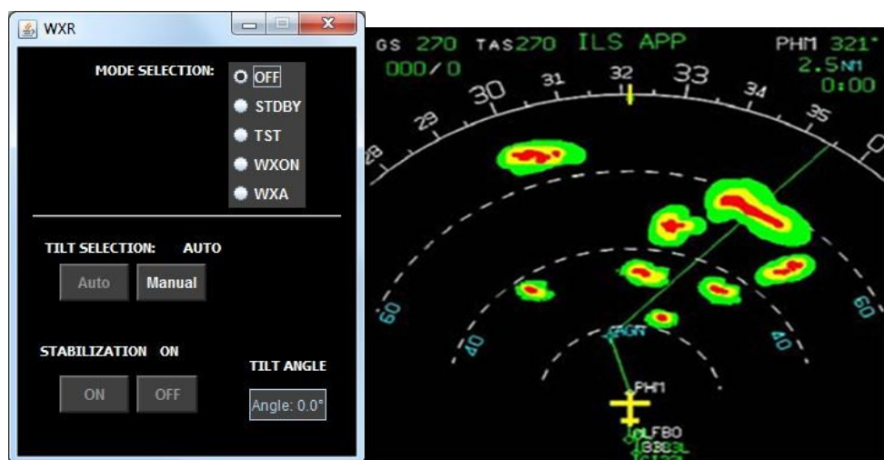
a) Weather radar control panel
