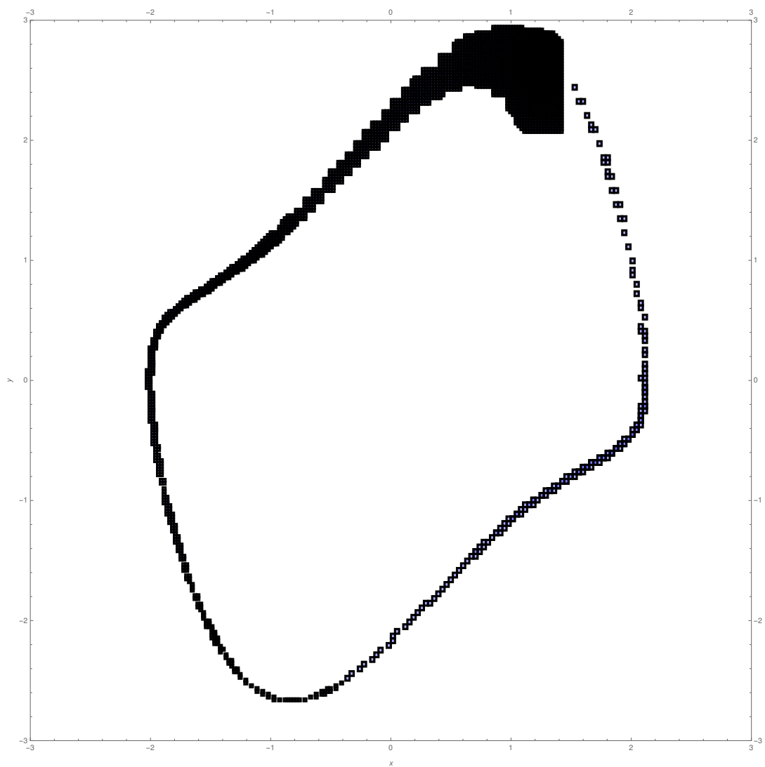
Figure 7.15 – The set obtained after using our CP Algorithm on every new Taylor model (6 order) evaluated at each time step over an interval [0, 6.70] .
