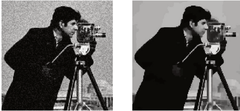
Figure 3.5 – Denoised version (right) of a noisy image (left) obtained through the Sinkhorn-like algorithm I.4
