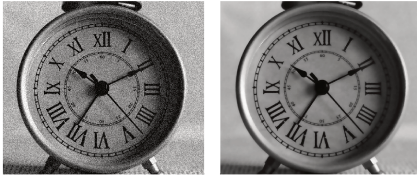
Figure 10.1 – Denoising experiment using the ROF model with TV_{RT}^h : on the left, the noisy image g^h ; on the right, the denoised image \bar{u}^h
