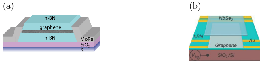
Figure II.2 – Structure of Josephson junctions reported in the literature, a low-Tc superconductor is deposited on top of a graphene sheet. (a) The superconductor MoRe is contacting a graphene sheet on the side, image taken from [?]. (b) The superconductor NbSe 2 is deposited on a graphene sheet, image taken from [?].
