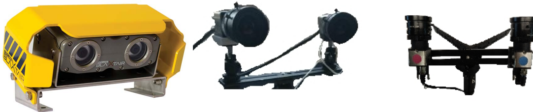
(a) Stereo camera mounted in to a rigid metal cage.
