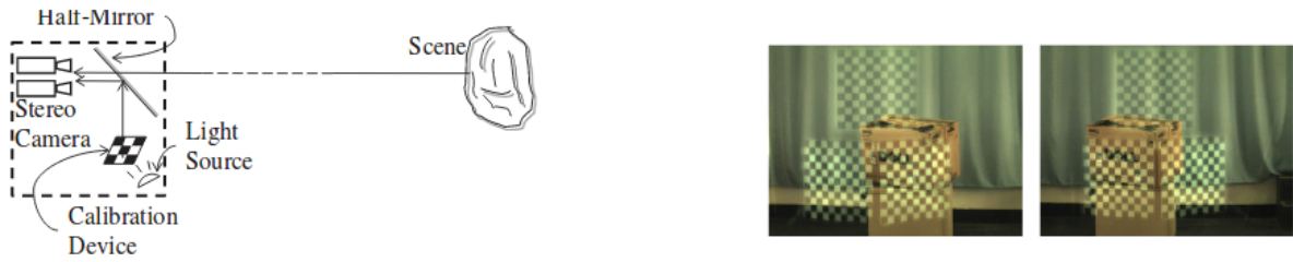
Figure 2.6: Embedded calibration stereovision system (left) and embedded stereo pair (right).
