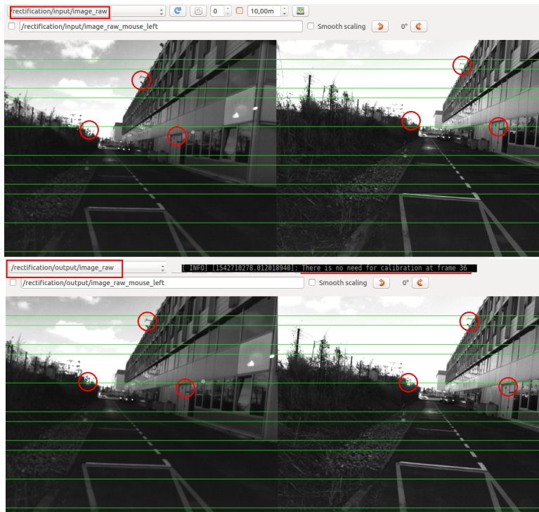
Figure 4.56: Rectification process realized on the extrinsic parameters which are based on the traditional method - it is realized on the first part of custom dataset.
