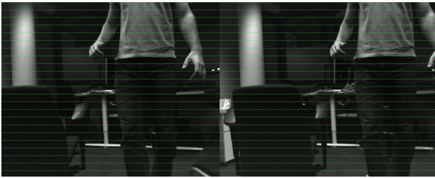
(a) Two views in co-planar plane, after rectification process. Green lines are epipolar lines.
