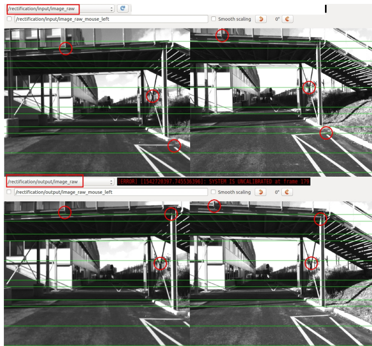
Figure 4.57: Rectification process realized on the extrinsic parameters which are based on the traditional method - it is realized on the second part of custom dataset.
