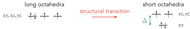
Figure 13.2 – Sketch of the effect of the structural transition on the t_{2g} orbitals in \text{Ca}_2\text{RuO}_4 .
