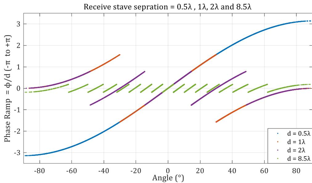
*Figure 25. Phase Difference between resulting Vernier pair of  $0.5\lambda$ ,  $1\lambda$  and Physical receiver pair separated by  $2\lambda$  and  $8.5\lambda$  as a function of angle of incidence. Vernier pair  $0.5\lambda$  is unambiguous.*
