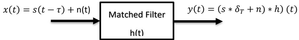
$n(t)$  is an additive noise term, and  $\delta_{\tau}$  is the delay operator.
