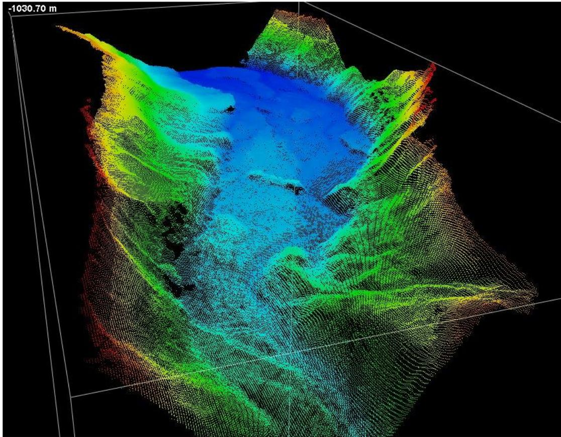
*Figure 3. Point-cloud view of a Digital Terrain Model (DTM) created using Bathyswath
