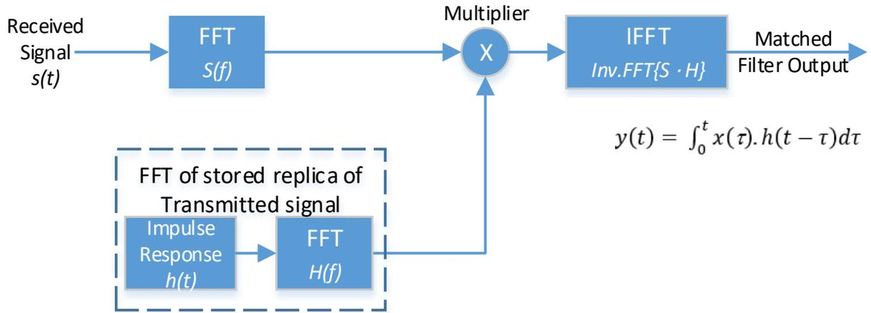
Figure 14 Matched Filter implementation using FFT
