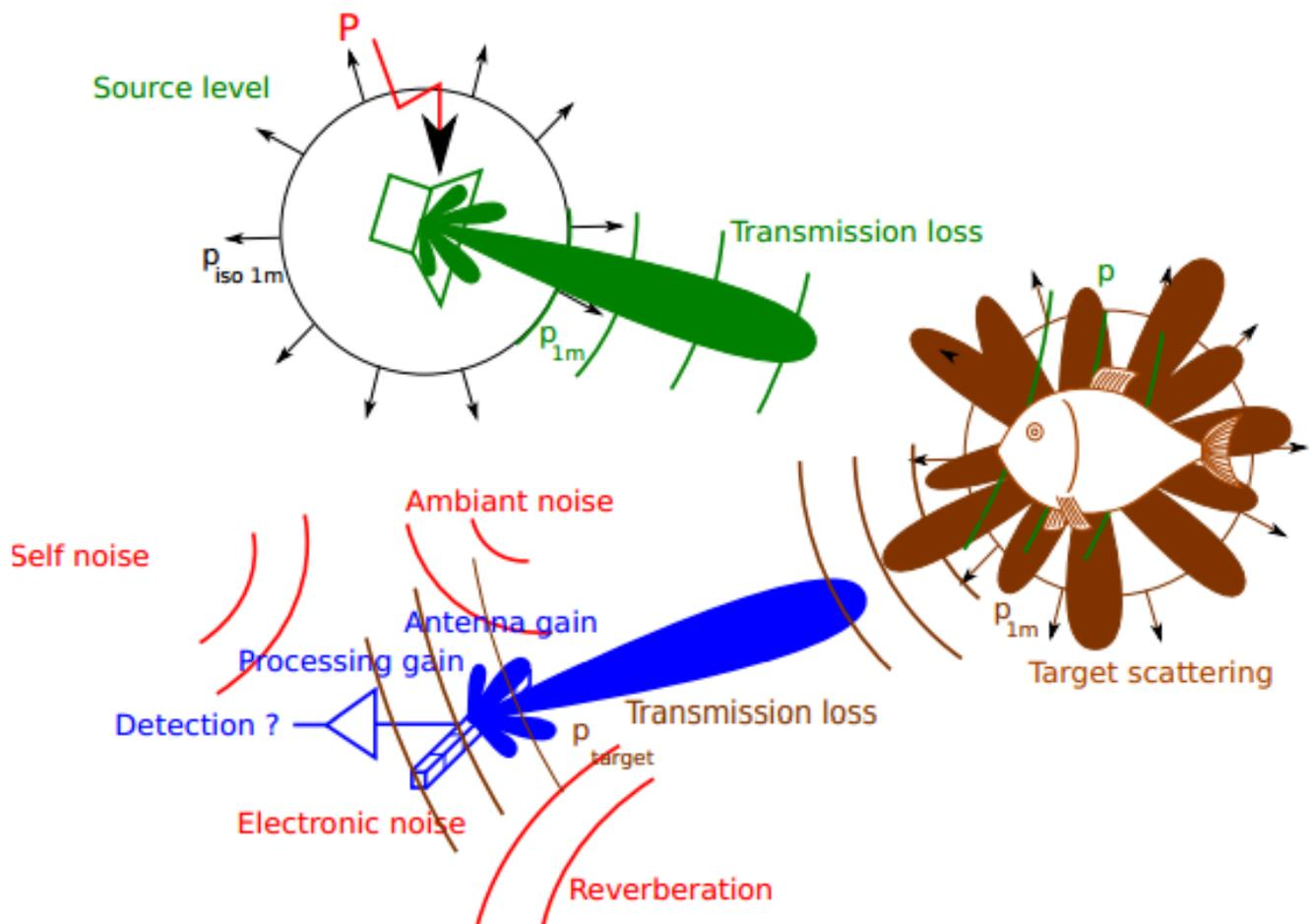
Figure 28 Sonar equation illustration for an active sonar
