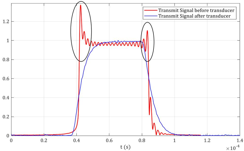
*Figure 61 Transmit pulse as input and output to piezoelectric*
