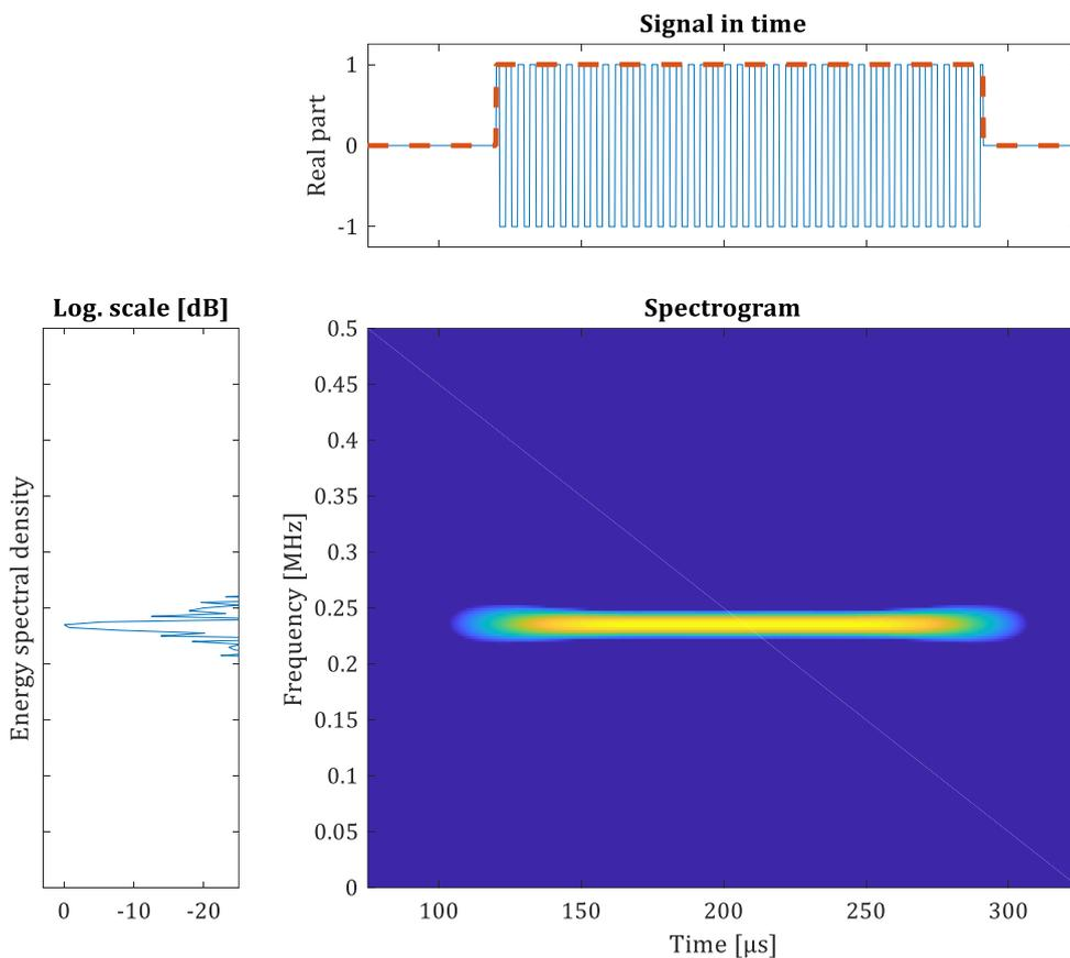
Figure 42 Spectrogram of CW signal with rectangular envelope
