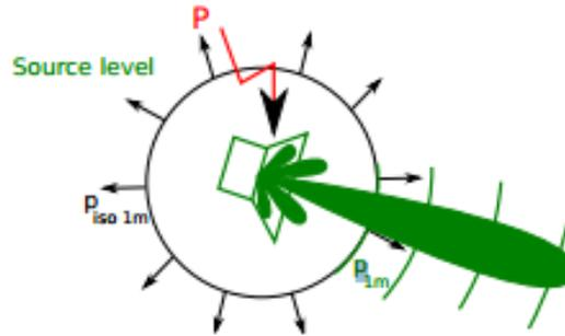
The source level is defined as the proportion of the measured pressure at 1-metre distance from the projector and a reference pressure.
