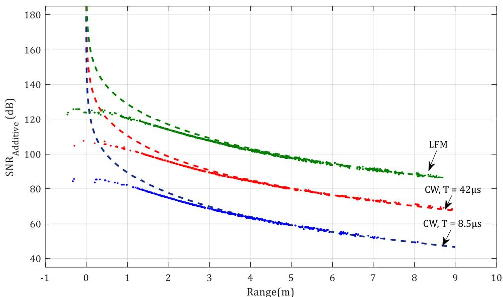
Figure 52 SNR accounting additive noise only, estimated for LFM (80 $\mu$ s), CW (8.5 $\mu$ s) and CW (42.75 $\mu$ s)
