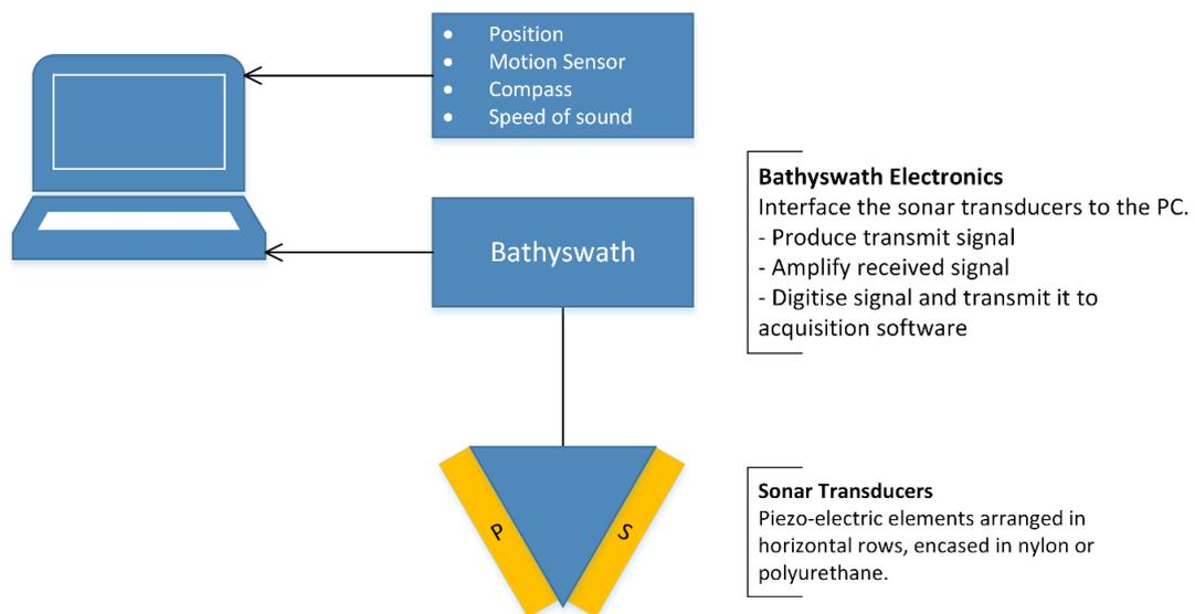
*Figure 9 Bathyswath System Setup*
