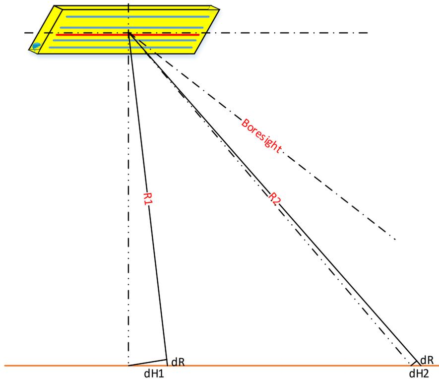
Figure 36 Measurement geometry in Nadir region
