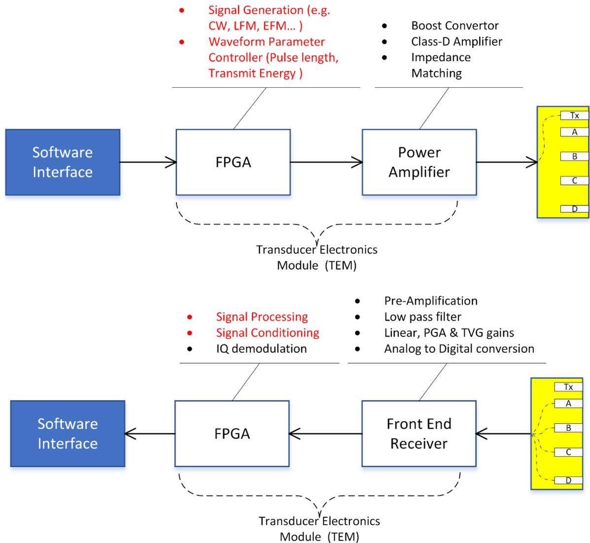
Figure 10 Bathyswath functional block diagram and the R&D works done in this thesis
