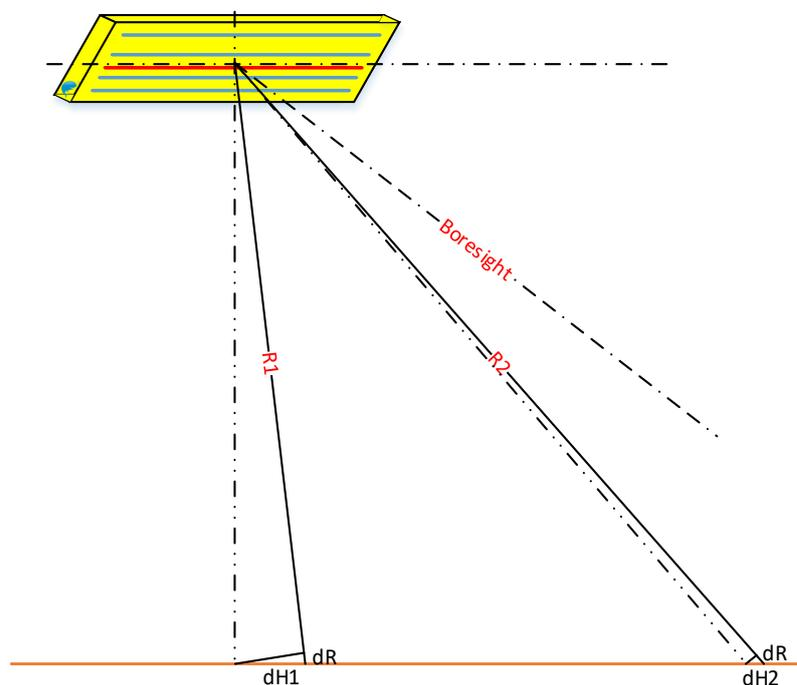
*Figure 71. Measurement geometry in nadir region*
