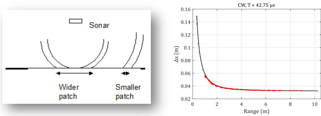
*Figure 72 Footprint patch in nadir region and far range (left), footprint length given over horizontal range*
