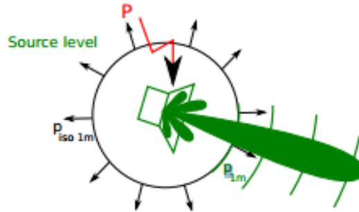
The source level is defined as the proportion of the measured pressure at 1-metre distance from the projector and a reference pressure.
