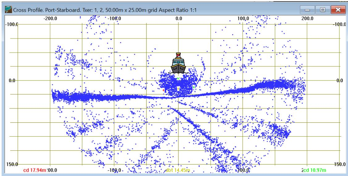
Figure 24 Depth vs horizontal range (Cross Profile), showing false bottom at different angles (picture taken during a test survey in Annecy lake with Boat setup)
