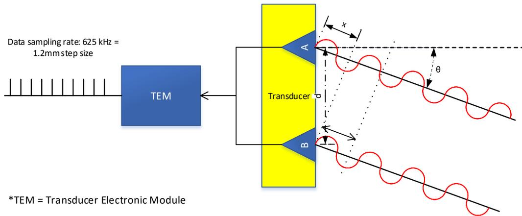
Figure 12. Basic setup of interferometry data acquisition
