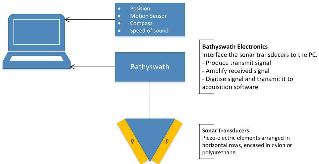
*Figure 9 Bathyswath System Setup*
