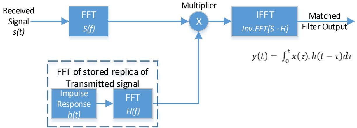
Figure 14 Matched Filter implementation using FFT
