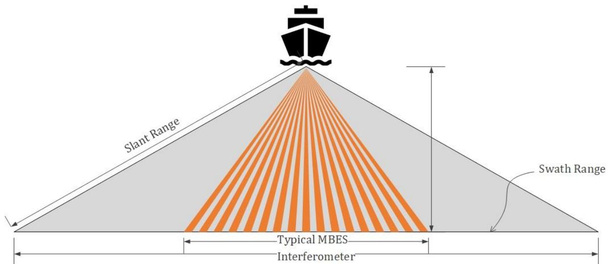
Figure 7. Interferometric vs Beamformer multibeam sonars [4]
