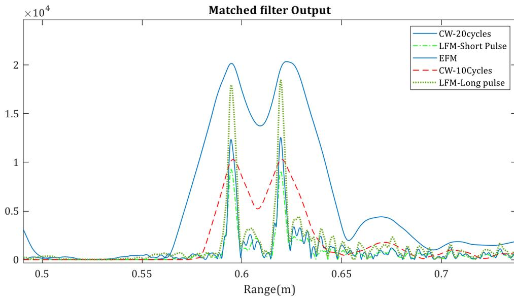
*Figure 51 Matched filter outputs with different transmit pulses*
