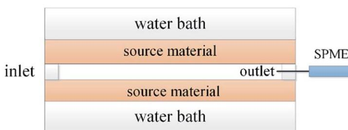
**Figure 19: A schematic representation of the improved sandwich-like chamber developed by Yang et al. [155]**
