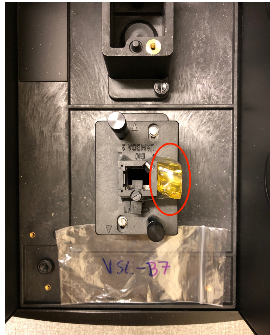
Figure IV.3: One of the 9 glass scintillators (in the red circle). The sample is placed in the same light spectrometer, in Fig. III.36, used for the \text{PbWO}_4 crystals.
