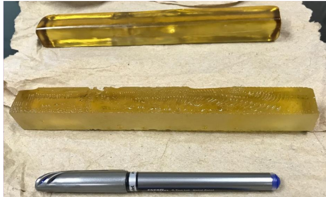
Figure IV.7: Glass scintillator size of 20 \times 20 \times 200 \text{ mm}^3 . Figure extracted from [113].
