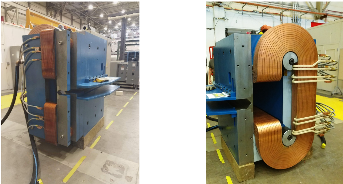
Figure III.4: Sweeper magnet. Left: front side of the magnet. Right: back side of the magnet.
