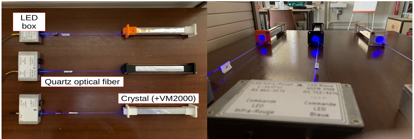
Figure III.45: Setup for optical transmission recovery via energy injection. Blue LEDs are being used in this picture. The recovery tests are done in the dark to reduce lights other than the LED light going to the crystal.
