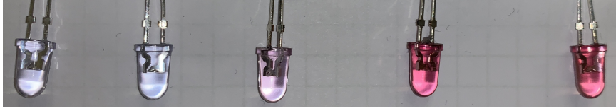
Figure III.44: Change of the color of the LED plastic enclosures. From left to right: without irradiation, 1.0 \times 10^3 Gy, 4.4 \times 10^3 Gy, 1.7 \times 10^4 Gy, and 1.5 \times 10^5 Gy of irradiation.
