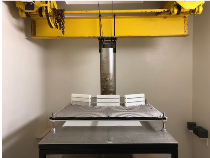
Figure III.31: Irradiation test facility in LCP. Nine sample boxes are positioned 60 cm away from the location of the ^{60}\text{Co} source. When the facility is not in use, the source is placed inside the tank at the bottom of the picture. When the test begins, the wires at the top of the picture pull out the source and position it at the center of the cylinder for the desired amount of time.
