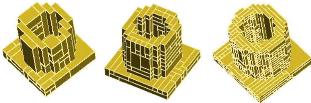
Figure 3.13: Mug representation using overlapping bricks. Three different minimum brick sizes are used.
