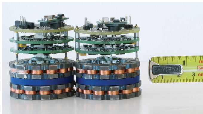
Figure 2.5: Planar Catoms V8 with solid state electronic controls at the top of the stack, sensors presented inside and electro magnets in orange color.
