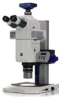
Figure 2.41 Le Microscope Axio zoom V16 (Zeiss).
