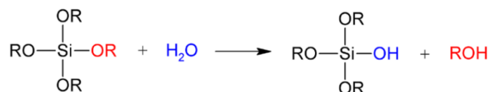
Scheme II-1: Hydrolysis reaction in the sol gel process of silicon alkoxide.
