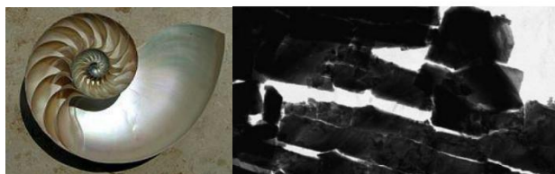
Figure II-18: Iridescent nacre in a nautilus shell (left) and TEM image of nacre platelets (right) [68].
