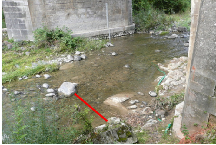
Figure B.17: Picture of the hydrometric station of Claduègne. The Red line locates the natural riffle controlling the stage-streamflow relationship at low flow. (picture taken from Tafasca (2017)).
