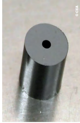
Figure 1.3 – Pellets of mixed oxides ( \text{UO}_2 and \text{PuO}_2 ) obtained after the manufacturing process. The pellets have a diameter and a height equal to 1 cm.
