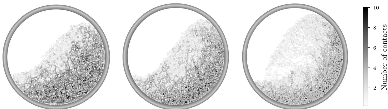
Figure 4.13 – Maps of particle connectivity after 13.75 rotations for \omega = 5.24, 7.85 and 10.47 rad/s. This snapshot corresponds to the instants 0.73t^*, 0.9t^* and 1.16t^* , respectively. The particle gray level is proportional to the number of contacts of the particle.
