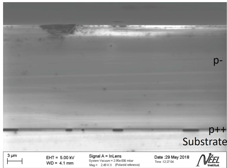
FIGURE 4.10: Polished side SEM picture, some cavities appear inside the p++ layer
