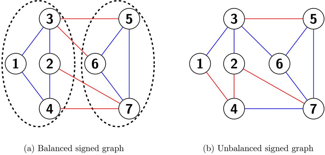
Figure 5.2: Example of a balanced (a) and an unbalanced (b) signed graphs. Negative edges are red while positive edges are blue.
