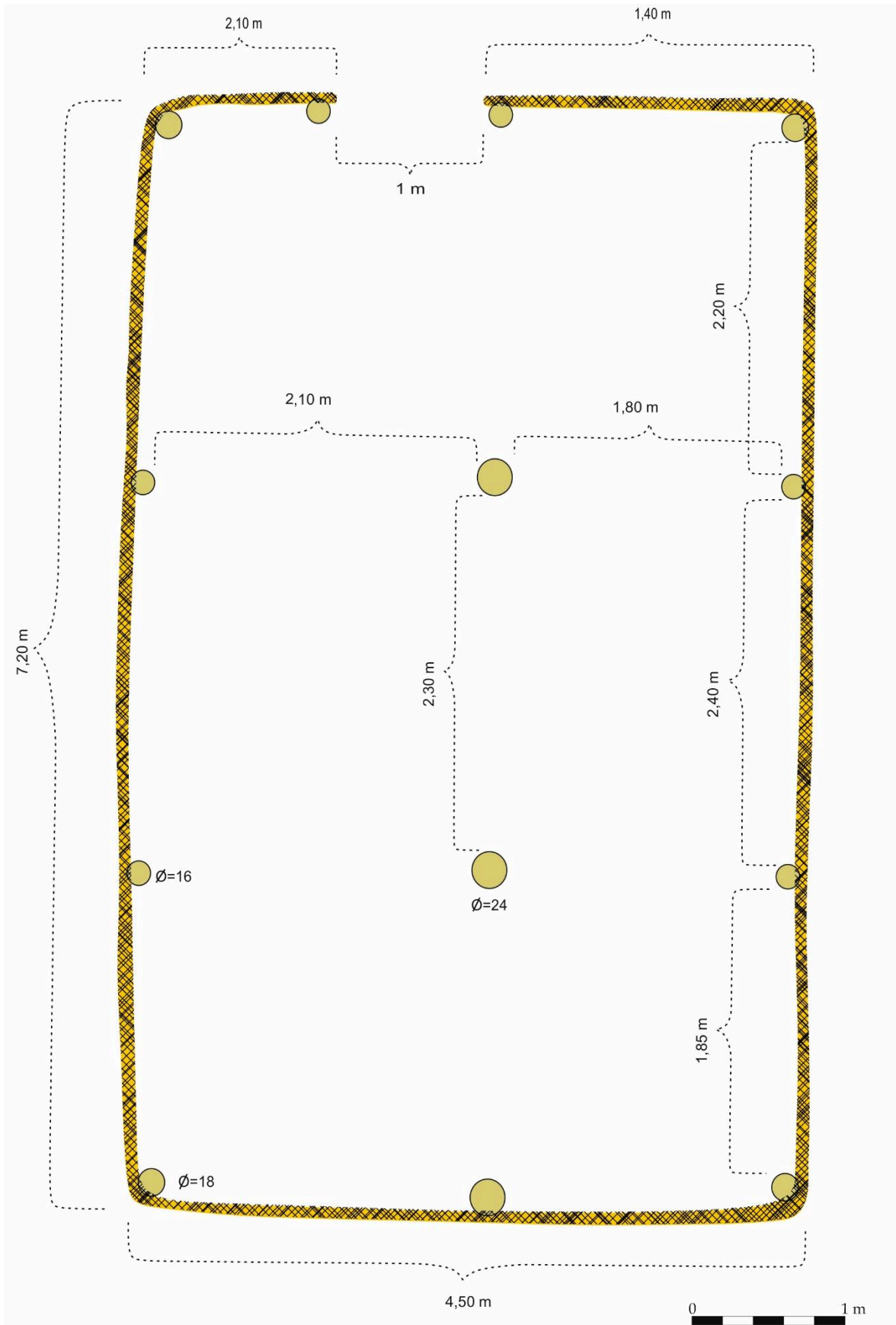
Figure 5.35: Wattle Structure: its plan with dimensions
