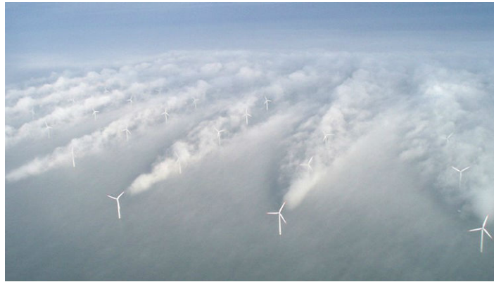
Figure 2.12 — Example of wake effect [57].
