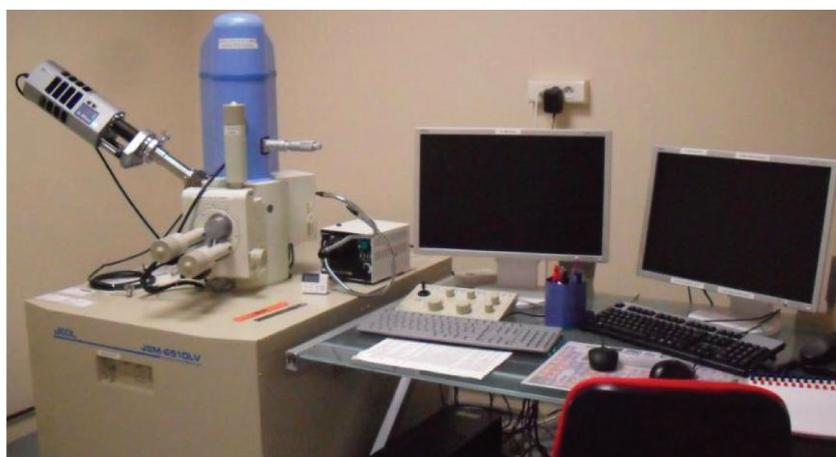
**Figure 2.7 Scanning electron microscope**
