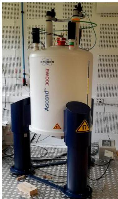
**Figure 2.16 NMR spectrometer**
