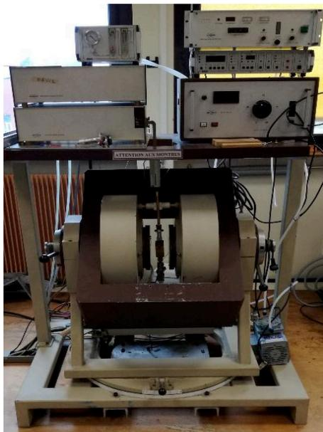
**Figure 2.14 Electron paramagnetic resonance spectrometer**
