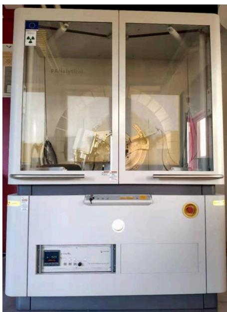
**Figure 2.10 PANalytical-Empyrean X-ray diffractometer**
