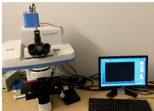
**Figure 2.12 XploRA Raman spectrometer from HORIBA Company**
