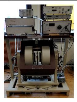
Figure 2.14 Electron paramagnetic resonance spectrometer
