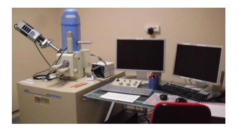
Figure 2.7 Scanning electron microscope
