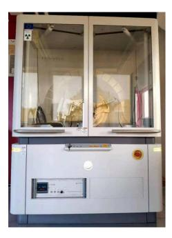
Figure 2.10 PANalytical-Empyrean X-ray diffractometer
