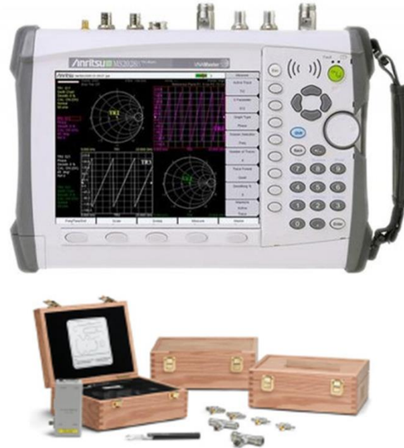
Figure B-2 Vector Network Analyzer ANRITSU-MS2026B and the calibration-verification kit.
