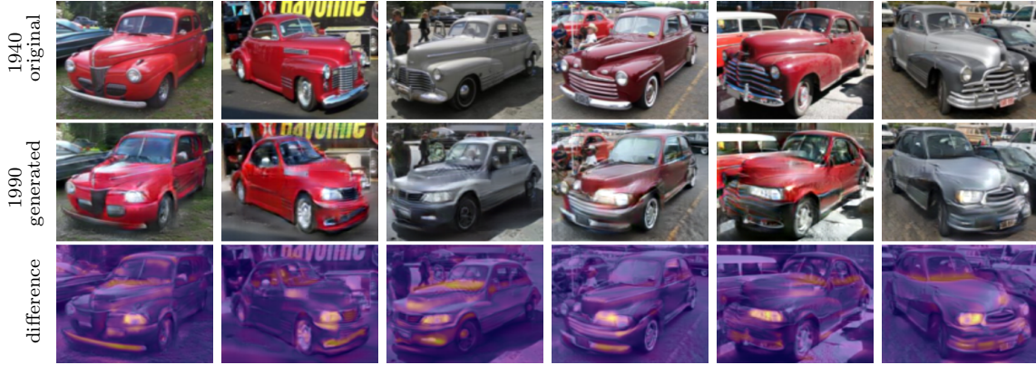
(b) Input images of cars from the 1940s (top row) and their generated translations into 1990s (middle row). In addition to the changes in the shape of headlights and the size of windows, similar to (a), the difference images (bottom row) highlight the disappearing metallic bumpers as well as the evolution of the shape of the hood, which flattens over time.
