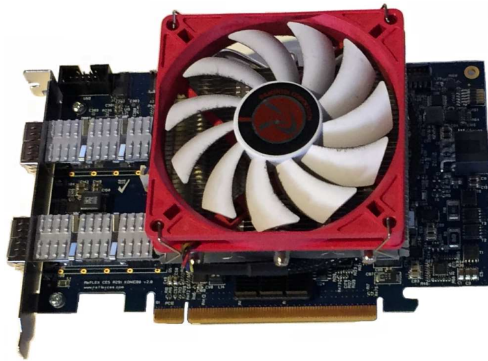
Figure 3.2: MPPA PCIe card [16]
