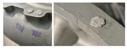
Figure 5.98: Examples of repaired cavity samples on a premium high-strength Al-Cu
