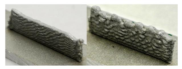
Figure 5.87: Single-track wall deposit by LMD of allow powder 224.0-A 80-100µm using parameters from trial 8 (left) and trial 5 (right)
