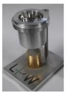
Figure 2.22: Standard Hall Flowmeter testing
