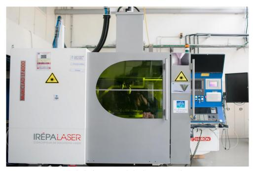
Figure 4.55: MultiCLAD LF4000 hybrid LMD manufacturing center
