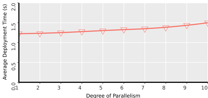
Figure 4.6 – Overhead of simultaneous container deployments.
