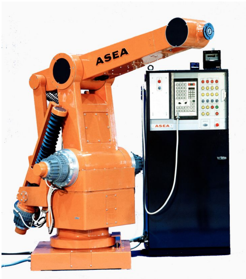
(c) ABB developed an industrial robot with a payload up to 60 kg in 1975 [IFR].
