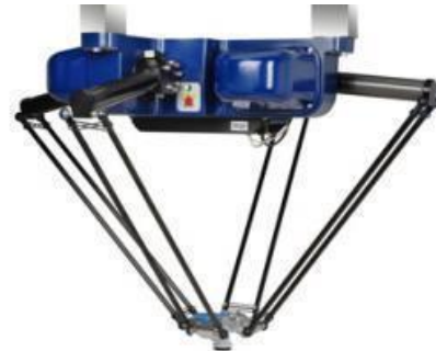
(b) H4 robot with asymmetrical design [Pierrot 2001].
