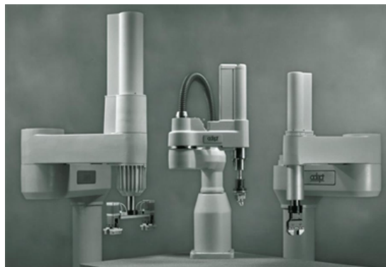
Figure 1.6: AdeptOne SCARA robot [Adept].
