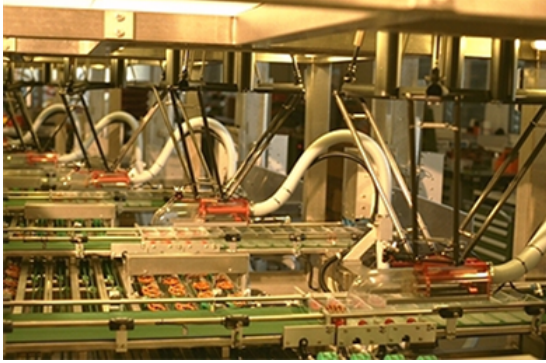
(a) Delta robots packaging pretzels [Bonev 2001].
