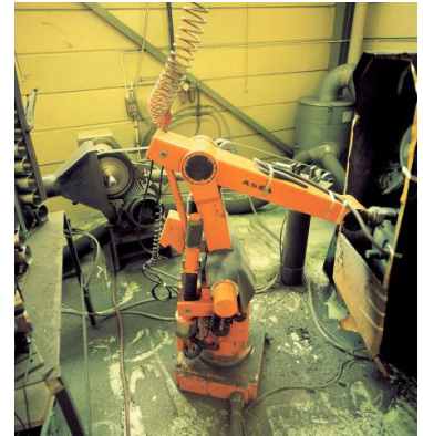
(b) The first fully electric robot, IRB 6 from ASEA in 1974 [IFR].
