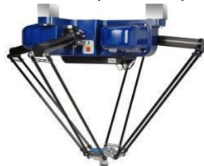
(b) H4 robot with asymmetrical design [Pierrot 2001].
