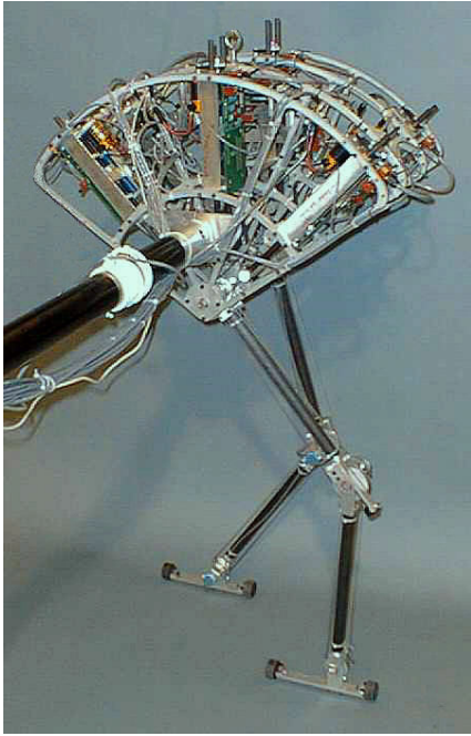
(a) Flamingo robot [Pratt 1998].
