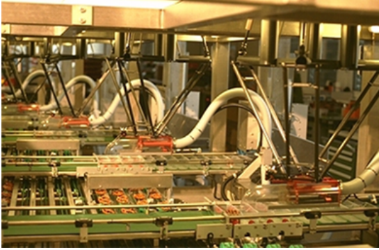
(a) Delta robots packaging pretzels [Bonev 2001].
