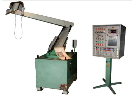
(b) First commercial painting robot in 1969 [IFR].
