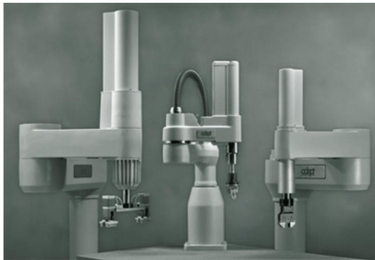
Figure 1.6: AdeptOne SCARA robot [Adept].
