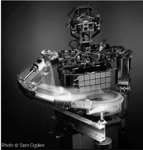
(c) Upper limb robot with SEAs [Brooks 1999].
