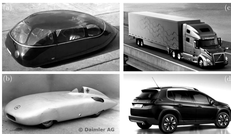
Figure 1.1: Typical old drag-optimized (a,b) and modern functionality-optimized (c,d) vehicle shapes illustrating the fundamental problem of vehicle aerodynamics being a trade-off between aerodynamic drag efficiency, aerodynamic stability and useful space. (a) Schlörwagen (1936). (b) Mercedes-Benz W125 Stromlinien (1938). (c) Volvo VNL (2017). (d) Peugeot 2008 (2019).
