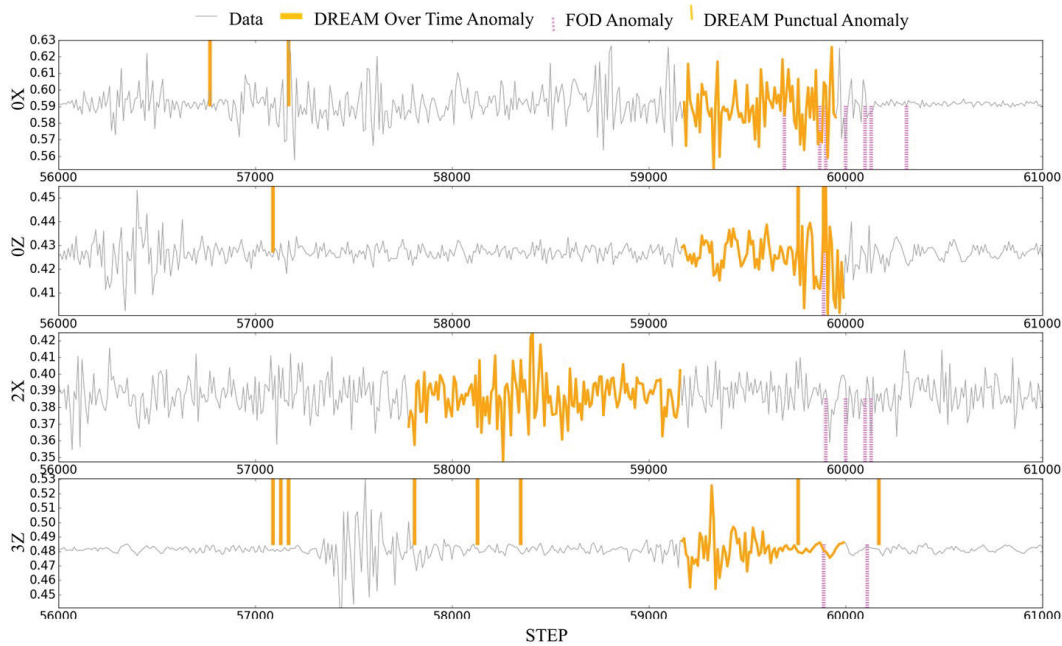
Figure 9.16 — Partial result of the Bridge Anomaly Detection.
