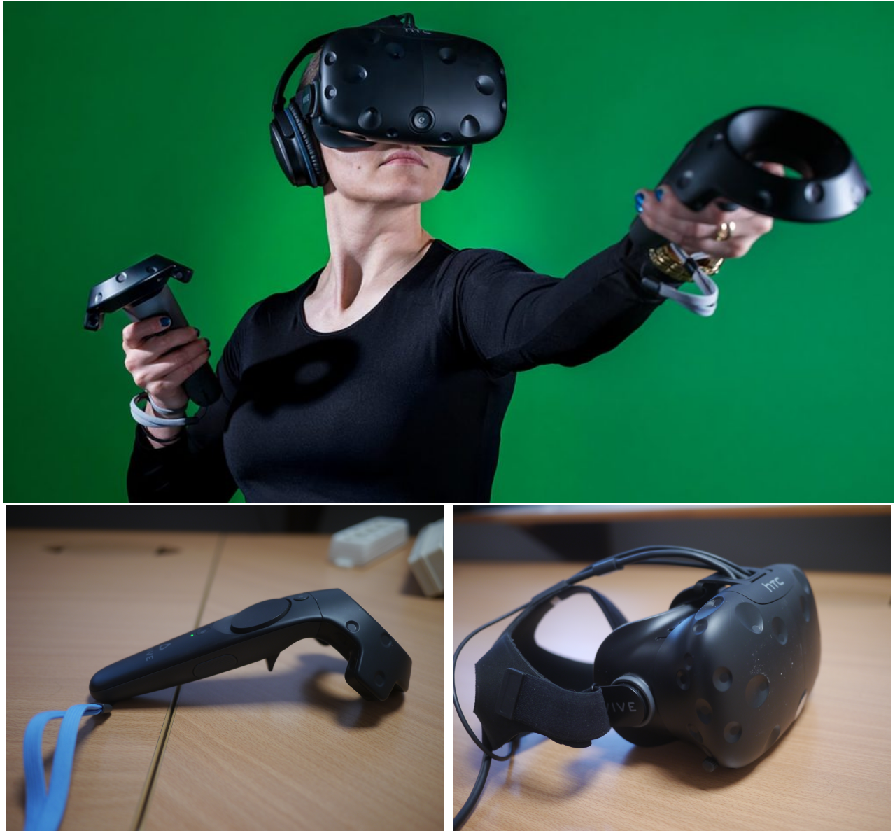
Figure 3.4: HTC Vive setup composed of two controllers and a HMD providing a stereoscopic display. The tracking is done at 90 fps at high precision.
