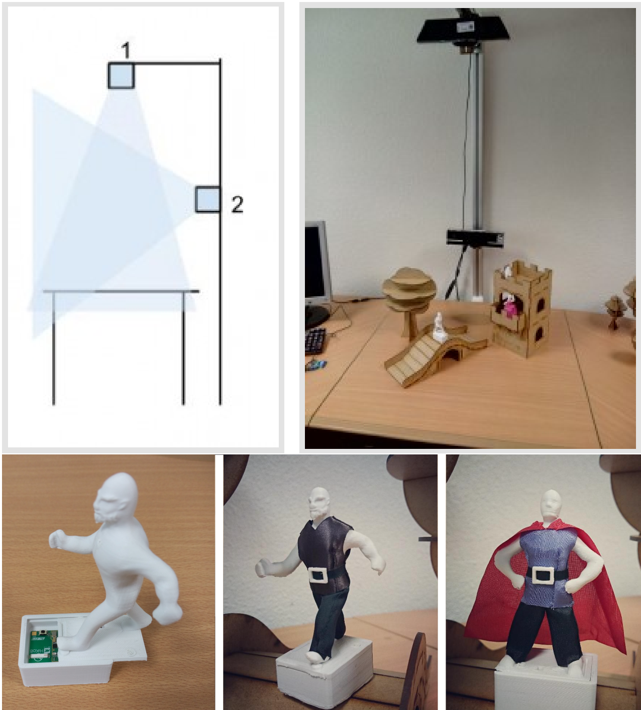
Figure 3.1: FIGURINES setup: figurines are tracked using a IMUs sensors paired with a top Kinect sensor. The frontal Kinect records the narrator’s facial expressions. The play stage is the table in the middle and covers a surface of 70 \times 70\text{cm}^2 .
