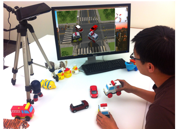
Figure 2.5: 3D Puppetry recording session. The user first scanned the figurines using the Kinect sensor to create corresponding textured 3D meshes. Figurines are then tracked in a real-time fashion using image-based feature correspondences and their rigid motion are transferred to the corresponding 3D models. We can notice that the user is provided with real-time feedback which is useful for making animation layers.
