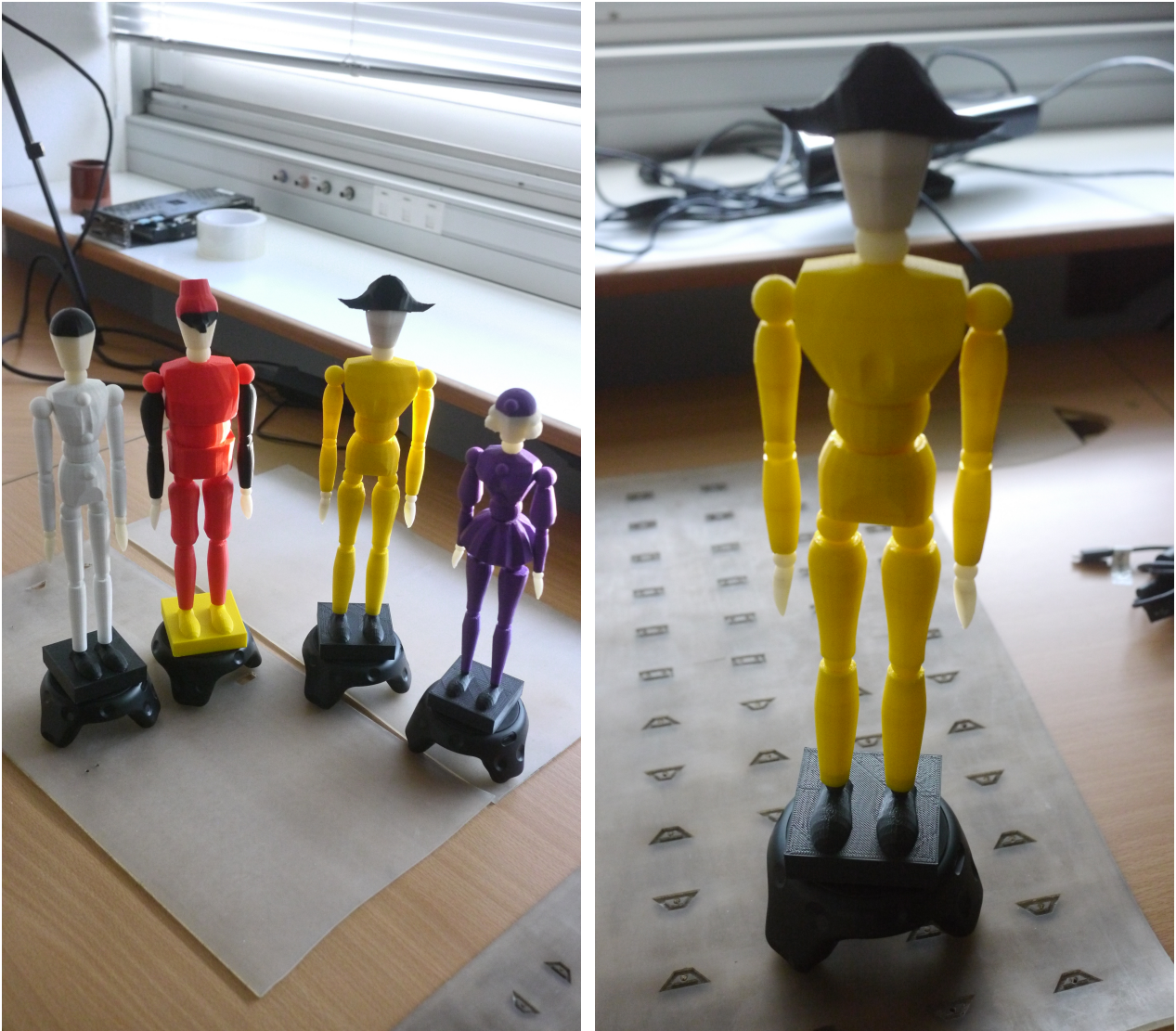
Figure 3.5: Commedia Dell'arte 3D printed figurines attached to HTC Vive trackers. For our experiment we printed a wood mannequin version of Arlequin, Pentalone, Pierrot and Colombine.
