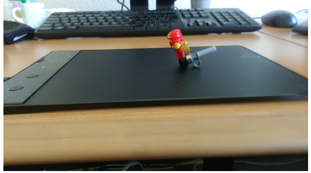
(b) We adapted the Slate 2 device by attaching the tracked ring to a LEGO brick.
