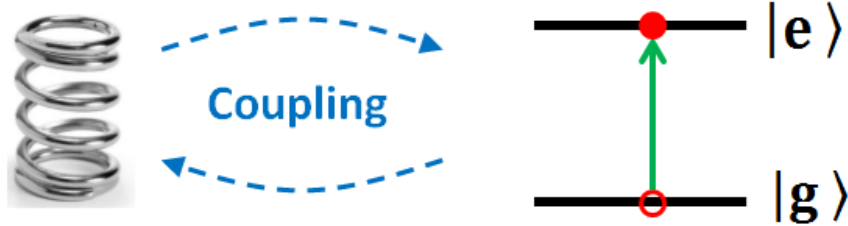
Figure 1.1: Quantum hybrid system: Coupling of a mechanical oscillator to a controllable quantum system.
