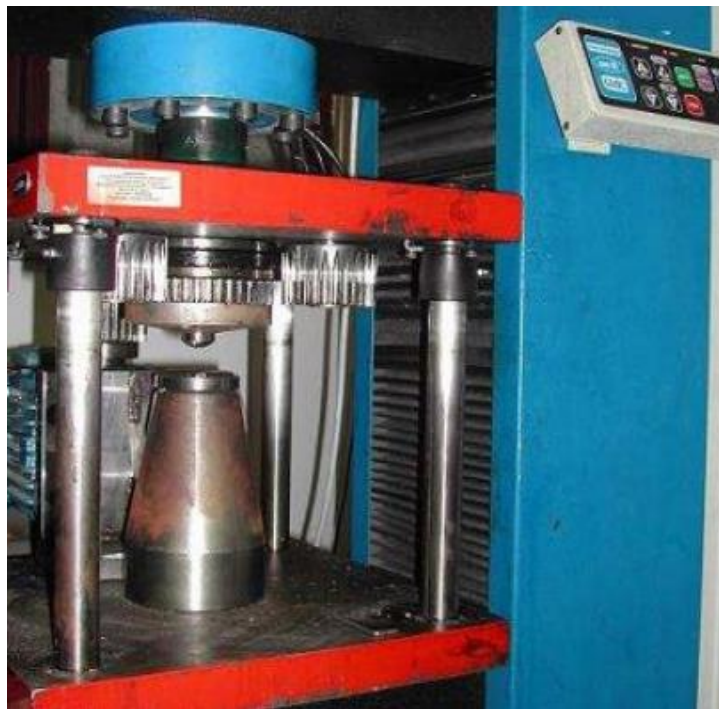
Figure 15: Universal Testing Machine EMIC and HPT accessory.
