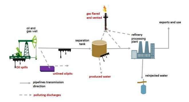
**Figure 3.** Upstream and midstream crude oil production chain. Oil is produced by extracting techniques at oil wells, then muds and residues are collected in pits, the oil and gas are transported via pipelines to separation batteries where oil, gas and produced water are separated. Crude oil is transported to refineries and to export ports. This process is not exempt of accidental or intentional discharges that can reach environmental compartments.
