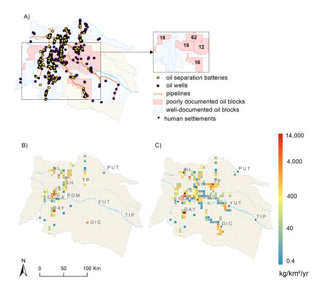
**Figure 10.** Spatial variations in oil spills during the T3 management period (2001-2011). (A) Map of the NEA showing the main oil infrastructures with well-documented (blue) and poorly-documented (red) oil blocks. (B) Originally recorded spills. (C) Harmonized map plotting data from (B) for well-documented oil blocks and average constant allocation to poorly-documented oil blocks.
