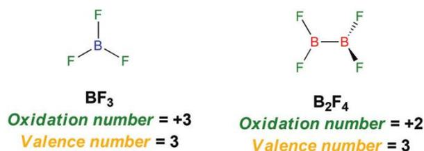
Figure 6. Differences in oxidation and valence numbers for  $\text{BF}_3$  and  $\text{B}_2\text{F}_4$
