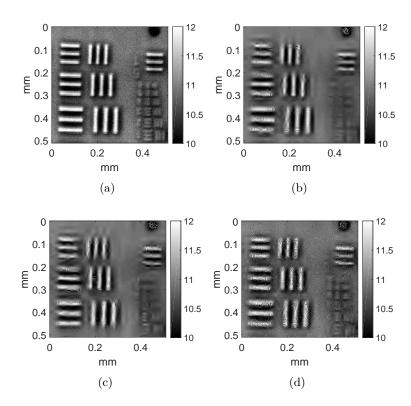
Figure 3.7: (a) Fully-sampled impedance (MRayl) map estimated from RF data acquired on the USAF 1951 resolution test chart, reconstruction results from Bernoulli random measurements for a measurement ratio of 0.25 with (b) proposed Cauchy-AMP, (c) ABE-AMP, (d) ST-AMP algorithms.
