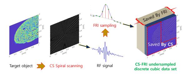
Figure 5.1: The block diagram describes the undersampling process based on the spiral pattern and FRI sampling in spatial and temporal domain respectively. The right cartoon clearly demonstrates the space saved by the proposed sampling scheme.
