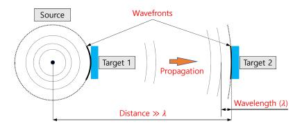
Figure 1.6: The target 1 receives a spherical wave whereas the target 2 located far away from the source experiences nearly a plane wave.
