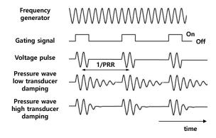
Figure 1.3: Generating pressure waves from electrical signals [Smith 2010]
