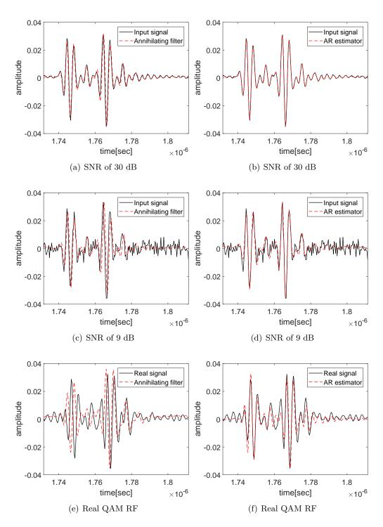
Figure 4.6: (a-d) Reconstruction results with AR model and annihilating filter method for a synthetic signal corrupted by an additive white Gaussian noise corresponding to (a-b) 30dB and (c-d) 9 dB, (e-f) reconstructed experimental QAM RF signal with AR-model and annihilating filter.
