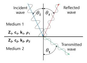
Figure 1.8: The dynamics of wave propagation occurring at the interface is illustrated.  $\theta$  indicates the angle between the travel path of the plane wave and the normal to the interface, and the subscripts i, r, and t stand for respectively incident, reflected, and transmitted.
