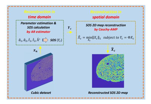
Figure 5.2: The block diagram describes the recovery process which is made up of two process, i.e., the parameter estimation in time domain and image reconstruction in spatial domain.
