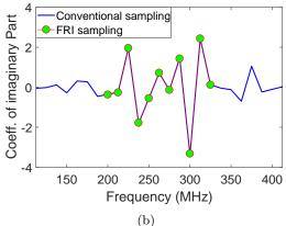
Figure 4.5: Real parts (a) and imaginary parts (b) of FT coefficients estimated from FRI sampling scheme (11 samples, *i.e.* 125 MHz) are overlapped on the FT coefficients acquired by conventional sampling (200 samples, *i.e.* 2.5 GHz).
