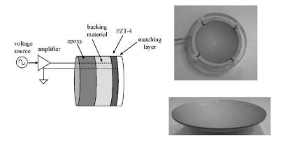
Figure 1.1: A single element transducer [Smith 2010]
