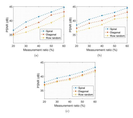
Figure 3.12: PSNR results as a function of the measurement rate, the sensing pattern (diagonal, random rows and spiral) and recovery algorithm (proposed Cauchy-AMP):(a), (b) and (c) are results of Cauchy denoiser with respect to respectively Human cornea at 500 MHz of SOS mode, Human lymph node at 250 MHz of SOS mode and Human lymph node at 250 MHz of impedance mode.
