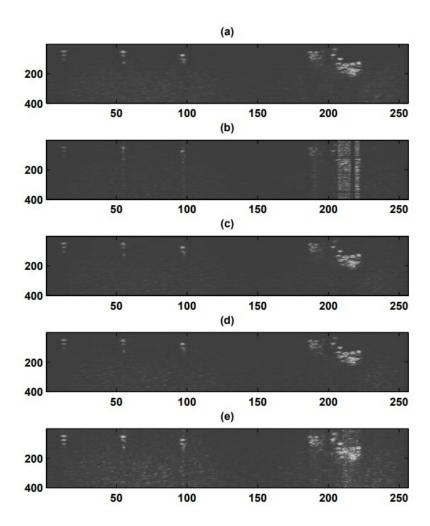
Figure 2.4: Comparison of original and reconstructed patches. (a) Original (RF) ultrasound image. Reconstructions with (b)  $\ell_{p_{opt}}$ -norm (c)  $\ell_{\alpha-0.01}$ -norm (d) BP and (e) OMP [Achim 2010].
