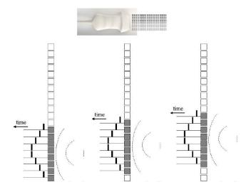
Figure 1.2: Electronic beamforming of a linear array [Smith 2010]
