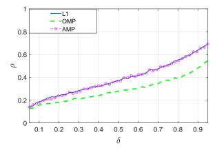
Figure 2.3: The phase transitions of reconstruction algorithms are compared.  $\delta$  and  $\rho$  denote the undersampling rate (M/N) and sparsity (K/N) respectively. AMP demonstrates the equivalent recovery performance to L1 reconstruction. AMP used in this simulation adopted the soft thresholding as the  $\eta$  function.
