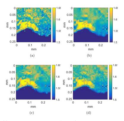
Figure 3.8: (a) Fully-sampled impedance (MRayl) map representing a reconstruction results from Bernoulli random measurements for a measurement ratio of 0.25 with (b) proposed Cauchy-AMP, (c) ABE-AMP, (d) ST-AMP algorithms.
