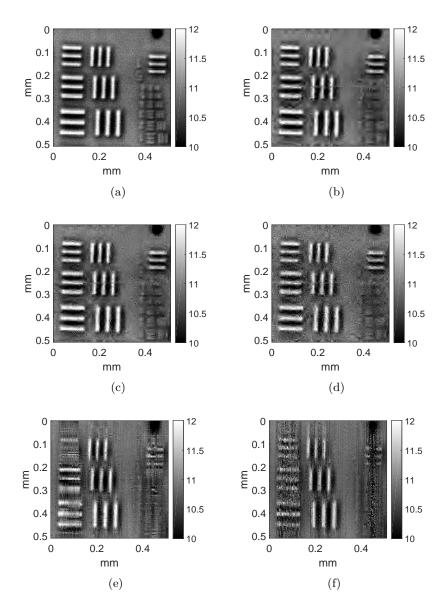
Figure 3.4: (a) Fully-sampled impedance (MRayl) map estimated from RF data acquired on the USAF 1951 resolution test chart, reconstruction results from Gaussian random measurements for a measurement ratio of 0.25 with (b) proposed Cauchy-AMP, (c) ABE-AMP, (d) ST-AMP, (e) IRLS and (f) L1LS algorithms.
