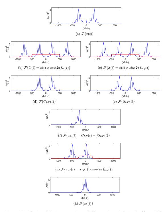
Figure 4.3: I-Q demodulation process is applied to an input RF signal x(t), and the resulting spectrum of the process is located on the baseband as shown in (h). The red lines indicate low pass filtering.
