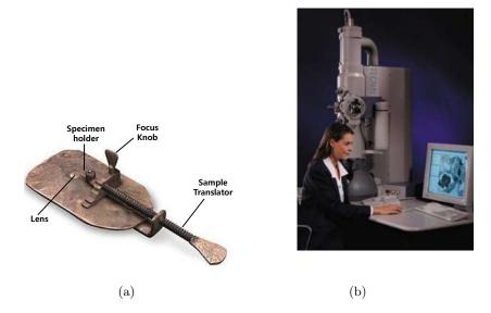
Figure 1.9: (a) Leeuwenhoek Microscope (circa late 1600s) of hand-held size acknowledged as the first practical microscope [Smith 2010], (b) Transmission Electron Microscopy (TEM) as one of the most advanced types of microscope [Alberts 2007].
