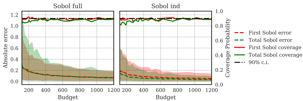
Figure 4.6 Variation of the absolute error and the POC with the computational cost for the RT method.
