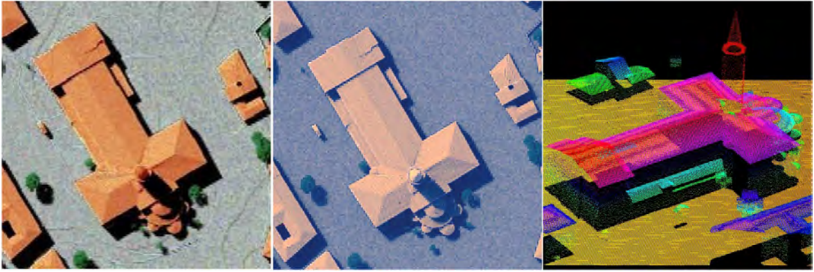
Figure 4.2: DART images of St. Sernin basilique (Toulouse). Radiometer: a) BOA, b) TOA, c) Airborne LIDAR (display with SpdLib software). Atmosphere: mid-latitude summer. Visibility = 23Km .
